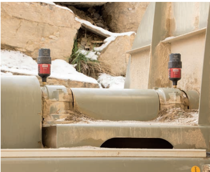
Industry: Quarry Application: Fan / blower bearings Lubrication system: perma STAR VARIO Installation solution: Direct mount
