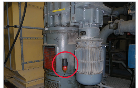
Lubrication of roller bearing on a mixer
