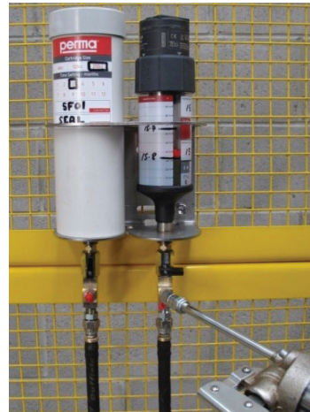
Fill grease lines with fresh grease using the manual purge valve or support flange
