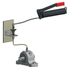
For remote mounting: Prefill lube-point and any grease lines / connections (use the same grease that is contained in the lubrication system)
